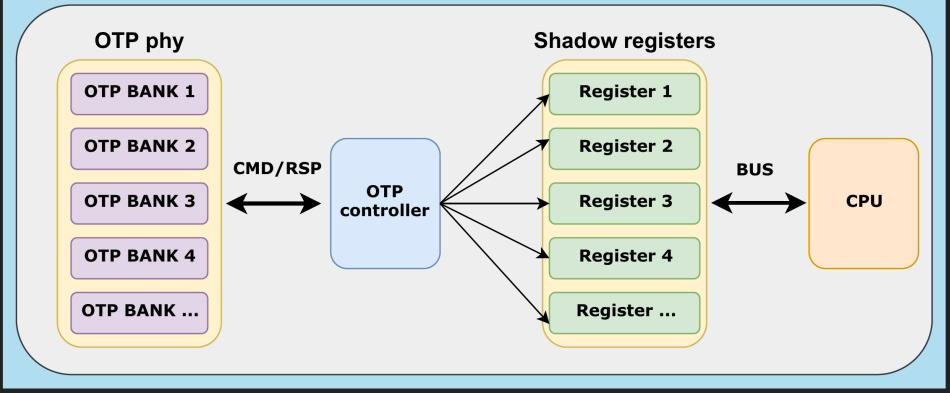
CPU is released from reset. Shadow registers can be read using system bus.
