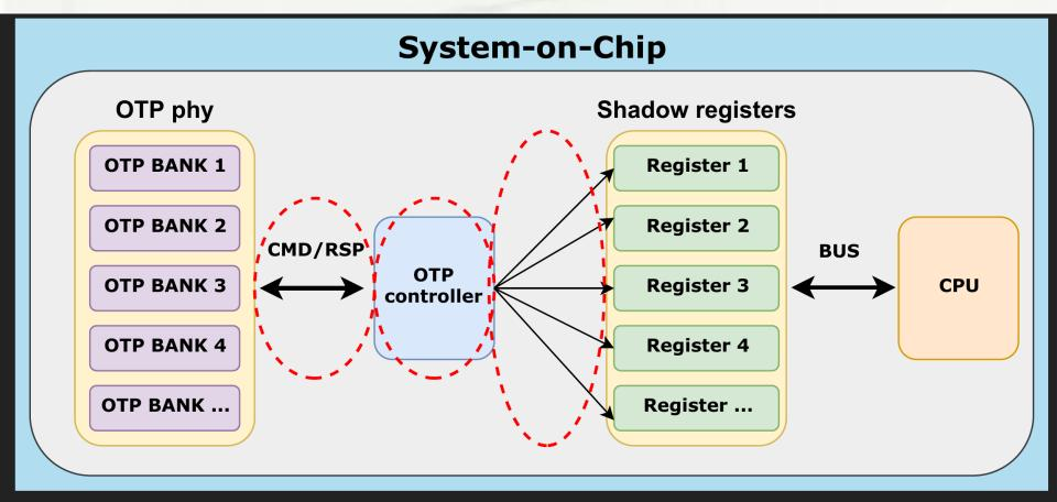
Attack the bus between the OTP controller and the shadow registers.
