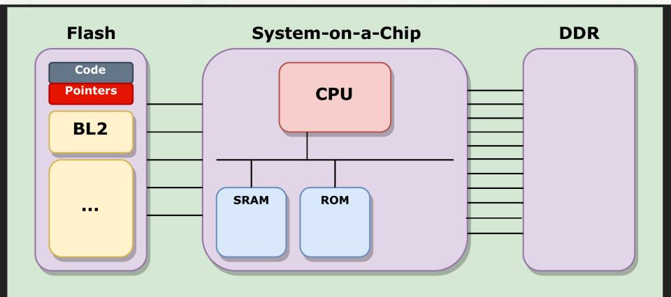
Replace encrypted BL1 with plain text code and pointers to SRAM.
