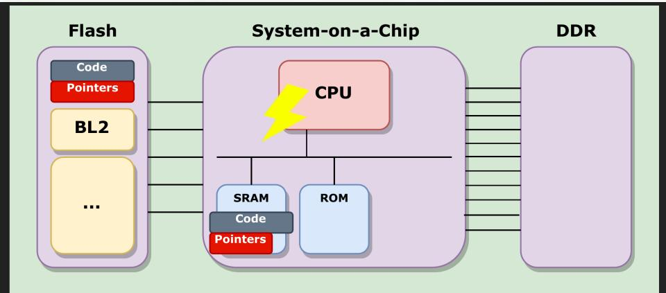
Glitch is injected after code copy and while pointers are being copied.
